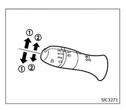
Move the lever up or down until the turn signal begins to flash, but the lever does not latch, and release the lever. The turn signal will automatically flash three times.
