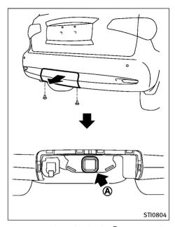
To access the trailer hitch  $(\widehat{A})$ , remove the trailer hitch cover located on the lower part of the rear bumper.
