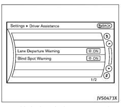
3. Highlight the "Blind Spot Warning" key, select ON (enabled) or OFF (disabled) and push the ENTER button (2).
