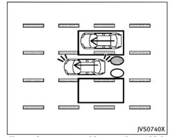
Illustration 5 - Overtaking another vehicle Illustration 5: If the driver activates the turn signal while another vehicle is in the detection zone, then the system chimes (twice) and the side indicator light flashes.
