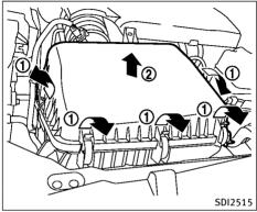
To remove the filter, release the lock pins  $\bigcirc$  and pull the unit upward  $\bigcirc$ .
