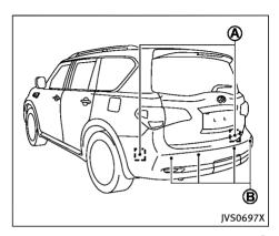
The BCI system uses radar sensors (A) installed on both sides near the rear bumper to detect an approaching vehicle and sonar sensors (B) to detect objects in the rear.
