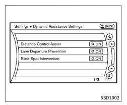
3. Highlight the "Distance Control Assist" key, select ON (enabled) or OFF (disabled) and push the ENTER button (2).
