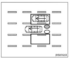
Illustration 9 - Entering from the side Illustration 9: If the BSI system is on and your vehicle approaches the lane marker while another vehicle is in the detection zone, the system chimes (three times) and the side indicator light flashes. The BSI system slightly applies the brakes on the appropriate side to help return the vehicle back to the center of the driving lane.
