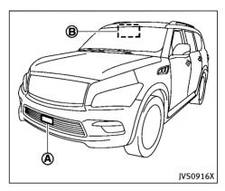
The FEB with pedestrian detection system uses a radar sensor (A) located behind the grille of the front bumper to measure the distance to the vehicle ahead in the same lane.
