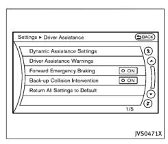
2. Highlight the "Forward Emergency Braking" key, select ON (enabled) or OFF (disabled) and push the ENTER button (B).
