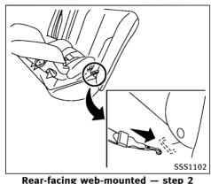
Secure the child restraint anchor attachments to the LATCH lower anchors.
