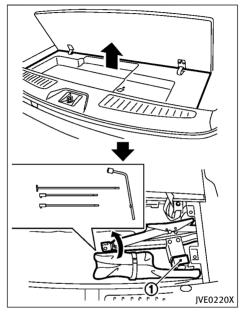
If rubber sound suppressor remains on jack when vehicle is being jacked up, the vehicle will be unstable and may fall off jack stand causing serious injury of death.
