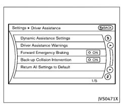
2. Highlight the "Back-up Collision Intervention" key, select ON (enabled) or OFF (disabled) and push the ENTER button (2).
