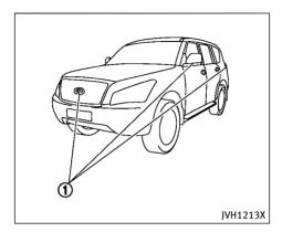
To display the multiple views, the Around View<sup>®</sup> Monitor system uses cameras ① located in the front grill, on the vehicle's outside mirrors and one just above the vehicle's license plate.
