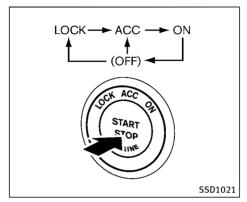
When the ignition switch is pushed without depressing the brake pedal, the ignition switch position will change as follows:
