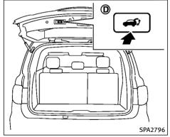
Power liftgate switch — Liftgate
