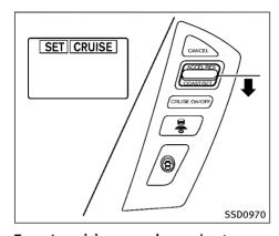
To set cruising speed, accelerate your vehicle to the desired speed, push the COAST/SET switch and release it. (The SET indicator will come on in the display.) Take your foot off the accelerator pedal. Your vehicle will maintain the set speed.
