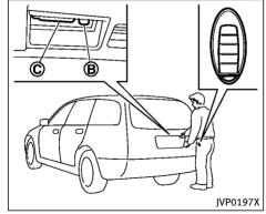
When you carry the Intelligent Key with vou, vou can lock or unlock all doors by pushing the door handle request switch (driver's or front passenger's) (A) or the liftgate request switch (B) within the range of operation.
