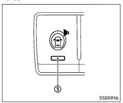
The warning systems switch is used to turn on and off the warning systems (Lane Departure Warning (LDW) and Blind Spot Warning (BSW) systems) that are activated using the settings menu on the center display.
