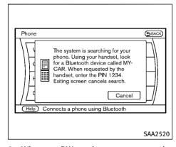
When a PIN code appears on the screen, operate the compatible Bluetooth<sup>®</sup> cellular phone to enter the PIN code.
