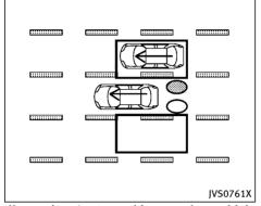
Illustration 6 - Overtaking another vehicle Illustration 6: If the BSI system is on and your vehicle approaches a lane marker while another vehicle is in the detection zone, the system chimes (three times) and the side indicator light flashes. Then, the BSI system slightly applies the brakes on the appropriate side to help return the vehicle back to the center of the driving lane.
