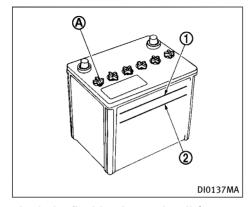
Check the fluid level in each cell (Remove the battery cover if it is necessary). It should be between the UPPER LEVEL ① and LOWER LEVEL ② lines.
