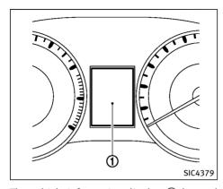
The vehicle information display ① located between the speedometer and odometer, and shows the indicators for the driving systems, Intelligent Key operation and various warnings and information.
