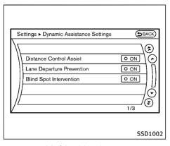
3. To enable/disable the LDP system, highlight the "Lane Departure Prevention" key, select ON or OFF and push the ENTER button (2).
